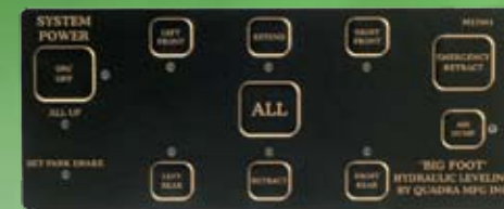
Manual Control Panel
